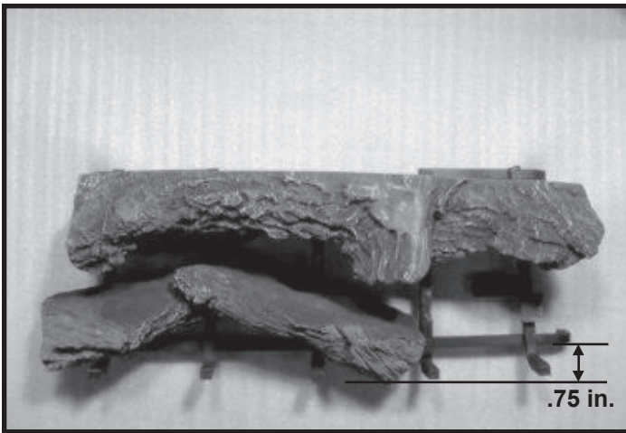
LOG NUMBER 2 (SRV768-704): Position log #2 onto grate such that tabs A and C fit into the slots on bottom surface of log. Slide the log all the way to the left. Then push the right front corner of the log forward until there is 0.75 in. between the front right corner of the log and the grate.
